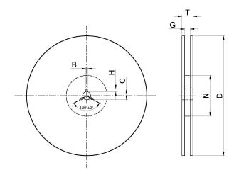
The beginning of the tape comprises a 200 mm long lead-in with vacant nests and at the hub end of the tape there are 10 to 20 sealed nests containing no devices .This end of the tap automatically detaches from the hub of the reel at the end of the inreeling procedure.
